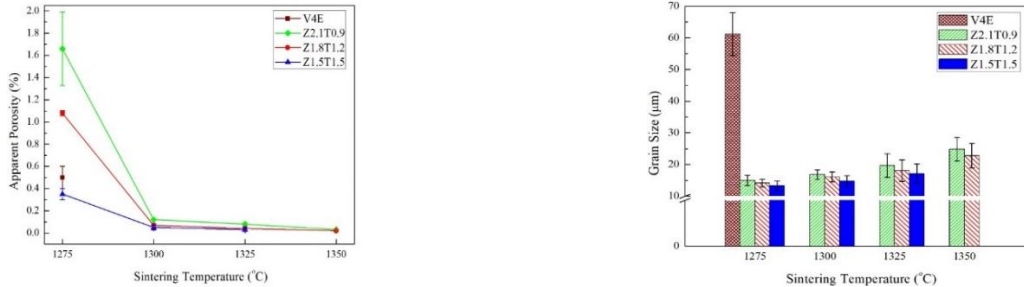
(a) V4 Extra-ZrC-TiC 之視孔隙率比較 (b) V4 Extra-ZrC-TiC 之晶粒尺寸比較
